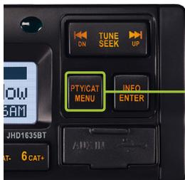
**PTY/CAT MENU:** Press & hold to enter menu. Press << or >> to navigate to SET CLOCK. Press ENTER to select. Press << or >> to adjust the HOUR. Press ENTER to move to the MINUTES. Press << or >> to adjust the MINUTES. Press ENTER to set the clock.
